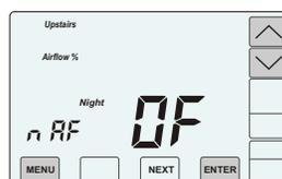
Touch the UP key to turn the option ON. Touch the DOWN key to turn the option OFF.
