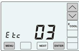
Touch the MENU key to display eCOOL TIMER option indicated by Etc. Touch the UP/DOWN keys to set the hours.
