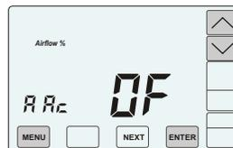
To turn Automatic Airflow Control OFF, touch the DOWN key. The user must set the airflow when automatic airflow control is off.
