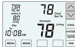
Touch the **UP/DOWN** keys to adjust the setpoint temperature. After 3 hours, the thermostat returns to the Schedule temperature.
